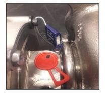
The seal number must be the one associated to the turbo number installed in vehicle.
